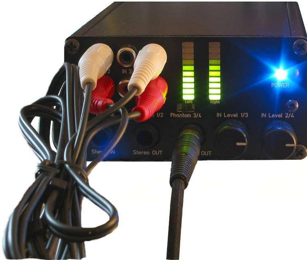
The picture above shows a loopback connection obtained by using the provided stereo RCA-RCA cable. The same connection can be obtained also by using a stereo JACK-JACK cable (connecting Stereo IN to Stereo OUT) or in other ways, for example using a stereo Jack to 2 RCA cable.
